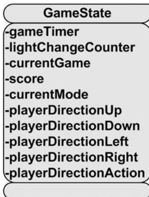
Figure 11-7. UML diagram of the GameState class
