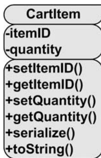
Figure 10-10. UML diagram of the CartItem class
