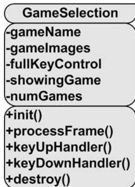
Figure 11-11. UML diagram of the GameSelection class
