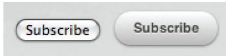
FIG 6.09: The default submit button in Safari on the left vs. one styled with CSS3—no images!—on the right.
